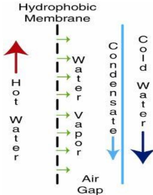
Figure-1, Air Gap type MD membranes
