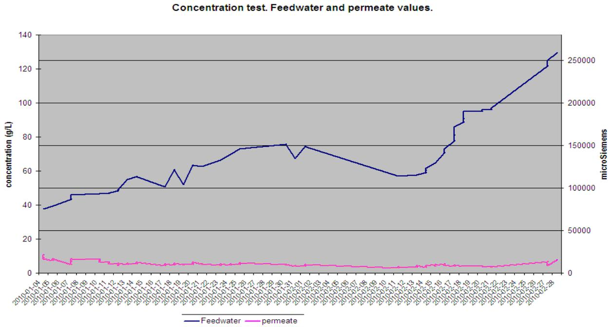
Figure. 7 Concentration test show conductivity (µS) during the test period January to end of Feb 2010.
