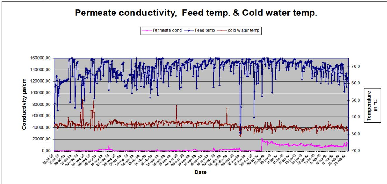
Figure 6 Permeate conductivity compared with temperature of feed and cooling water. The results of a final concentration test made during Jan-Feb 2010 are shown in Fig 7. As shown, the conductivity of the permeate is high (due to a leak) but relatively constant even at the end when
