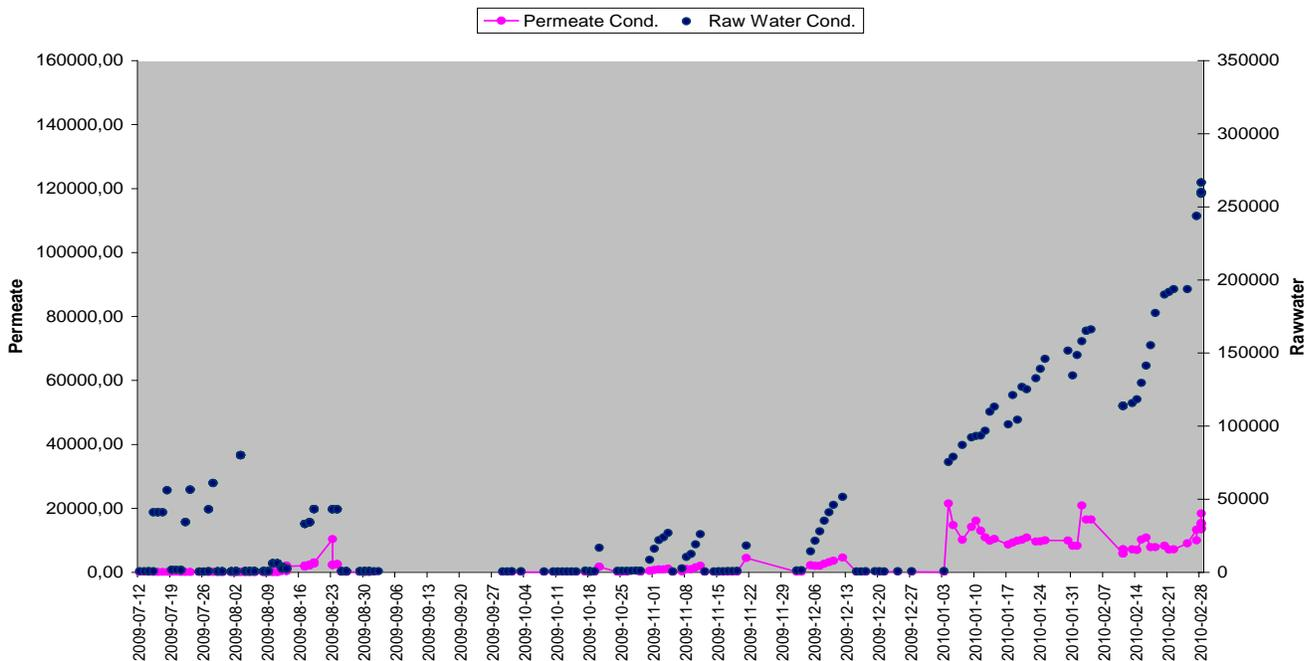
Figure -3 Permeate & Feed Conductivity Vs Time
