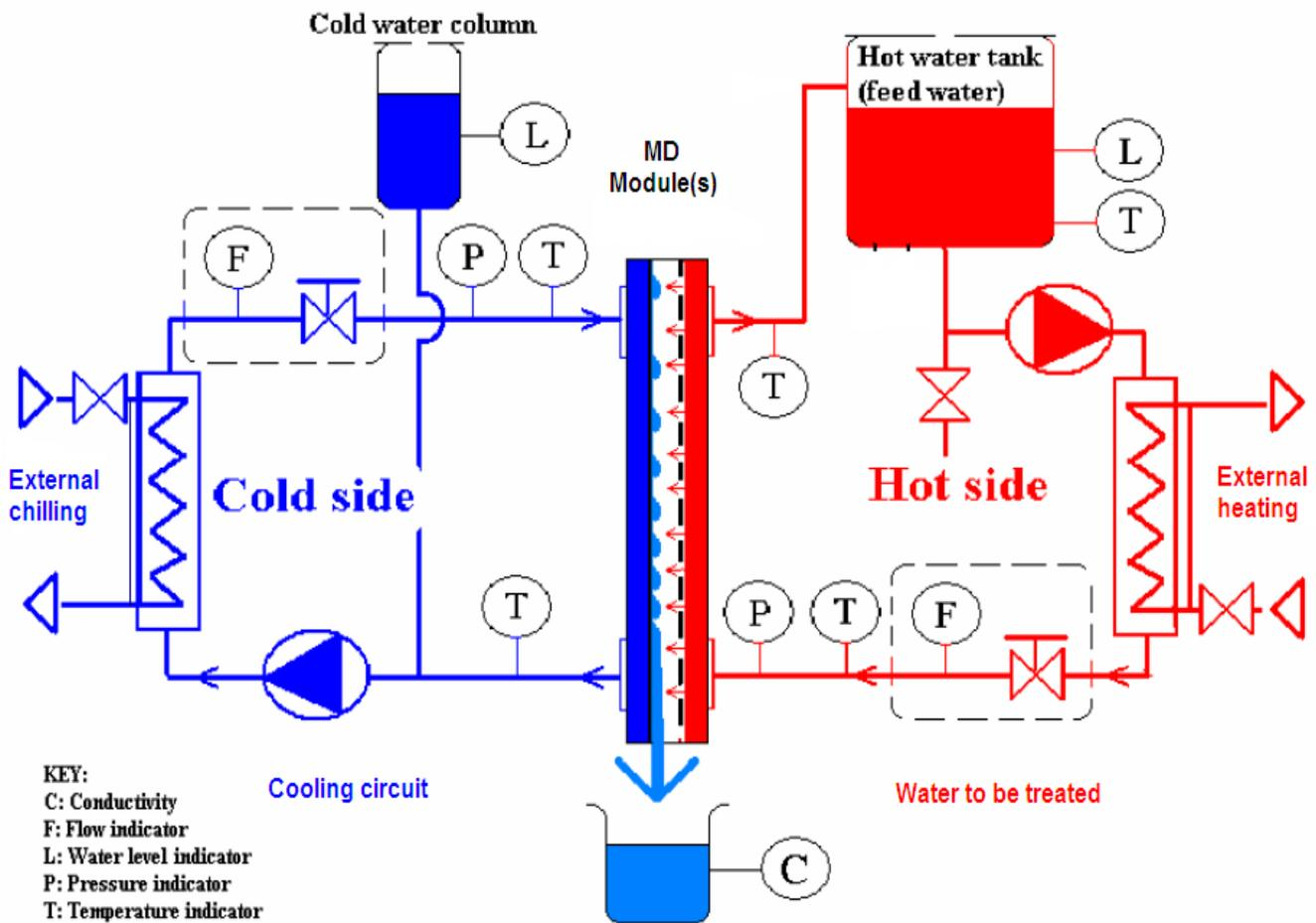
Figure- 2. Process flow diagram of the MD unit
