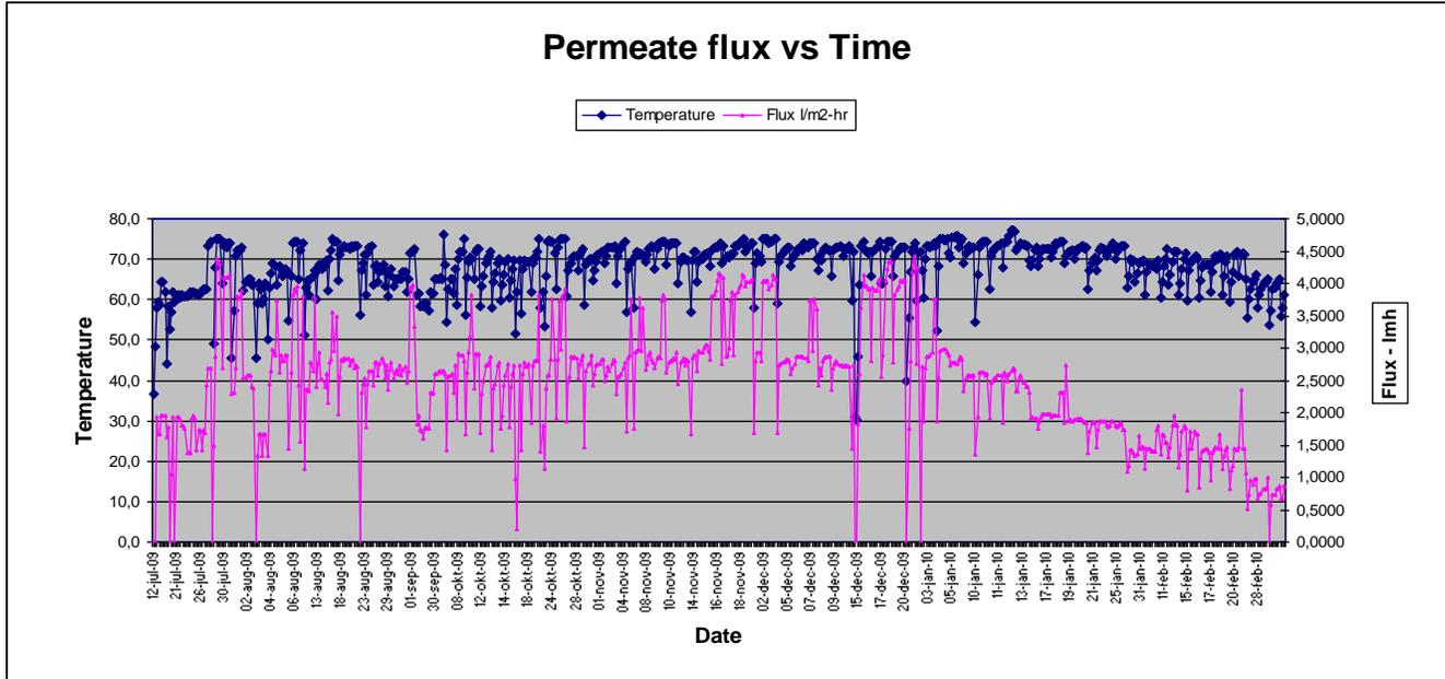
Figure. 5 Permeate flux compared with temperature over time
